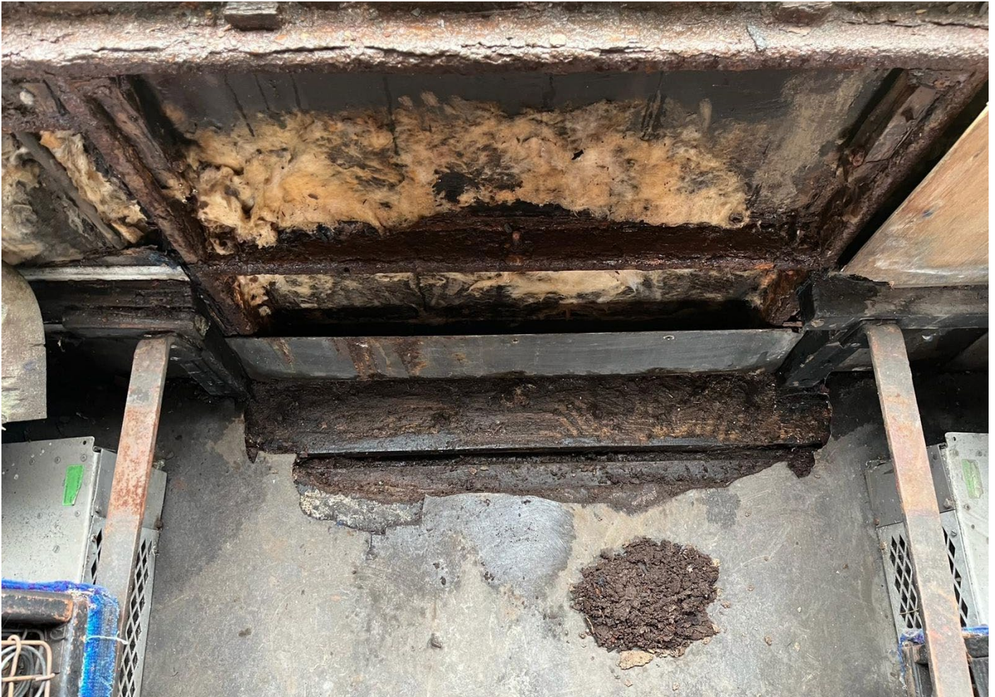
A picture inside 76275 showing where water has got in damaging the steel framework and the floor.
