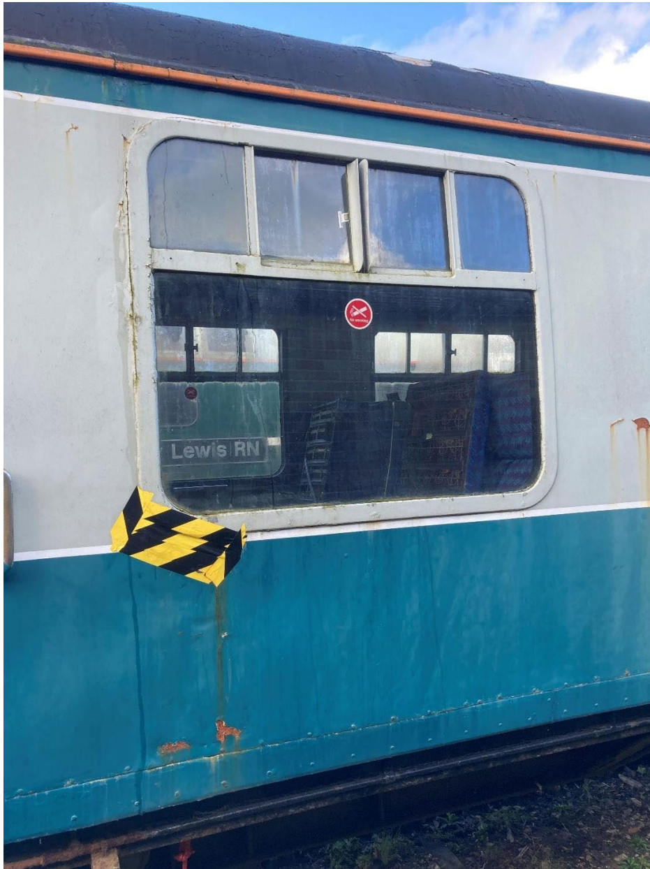
A couple of pictures of 76275 showing where the window frames have started to separate from the body allowing water in. This has then caused rust to appear below the windows causing holes on the outside, and damage on the inside which you will see on the next couple of pages.
