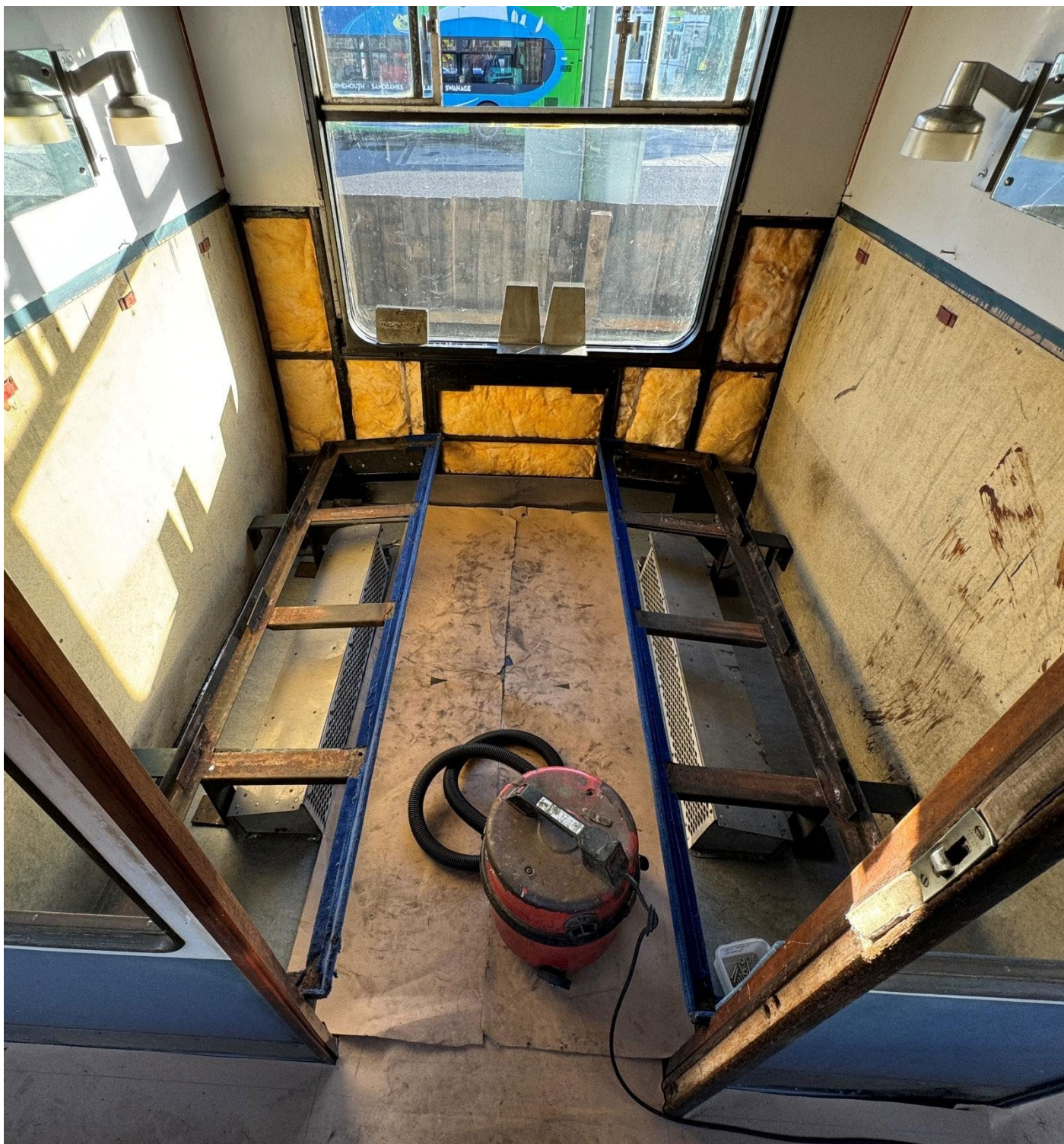
One of the compartments in 70824 showing work in progress with the heaters and seat frames refitted.
