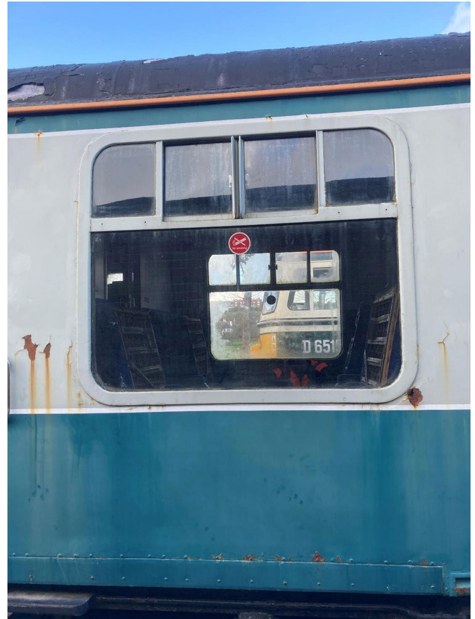
A couple of pictures of 76275 showing where the window frames have started to separate from the body allowing water in. This has then caused rust to appear below the windows causing holes on the outside, and damage on the inside which you will see on the next couple of pages.
