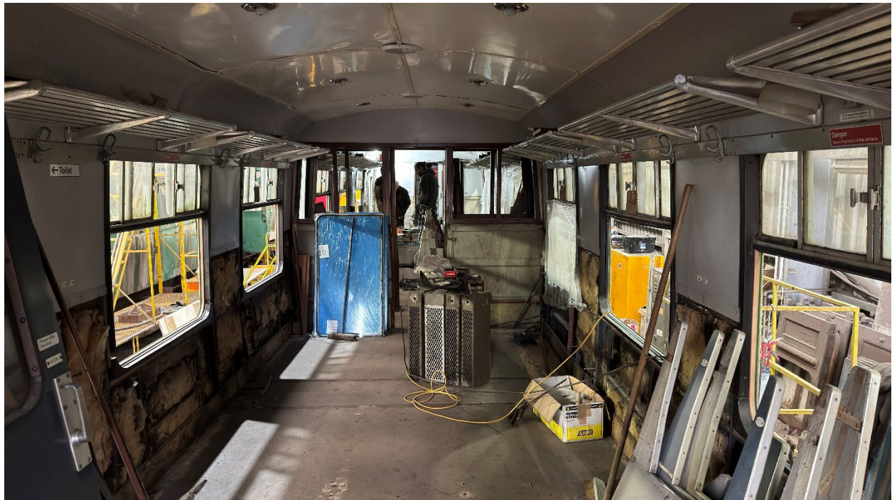
Pictures showing the extent to which the interior was stripped out for repair work to take place
