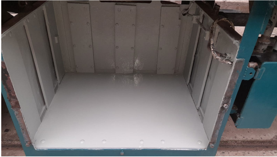
Battery box after rebuilding
