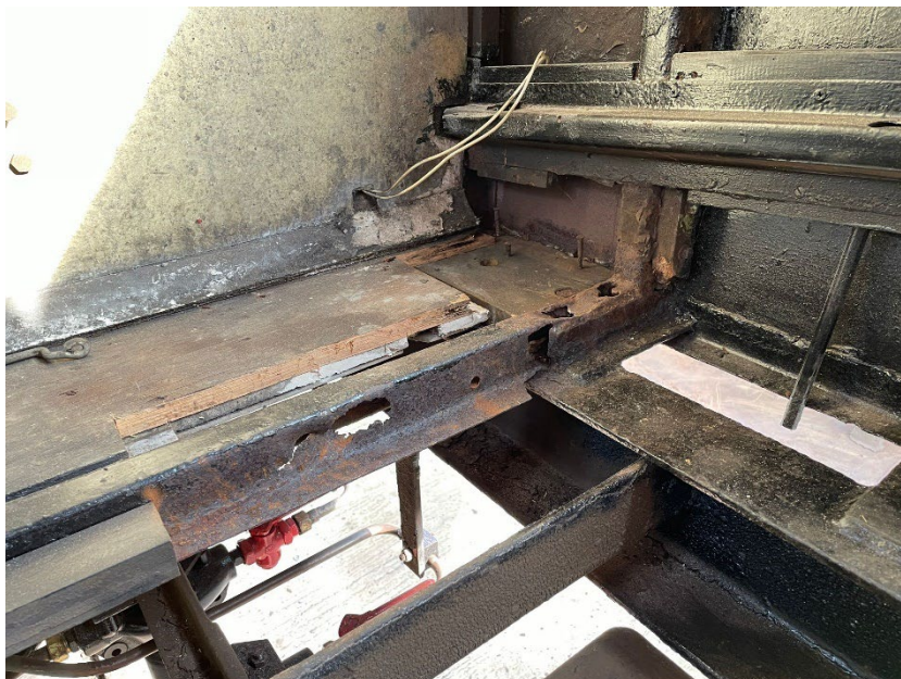
Before and after welding in new floor "top hat" support section
