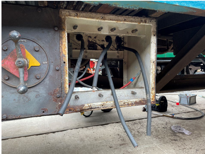
New ETH cables being run in to auxiliary supply case
