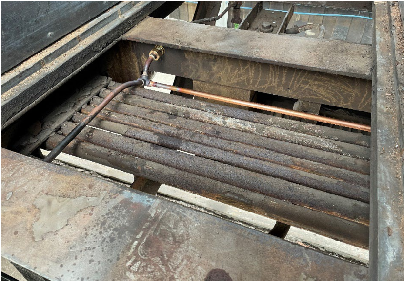
New brake pipework fitted to replace stolen sections
