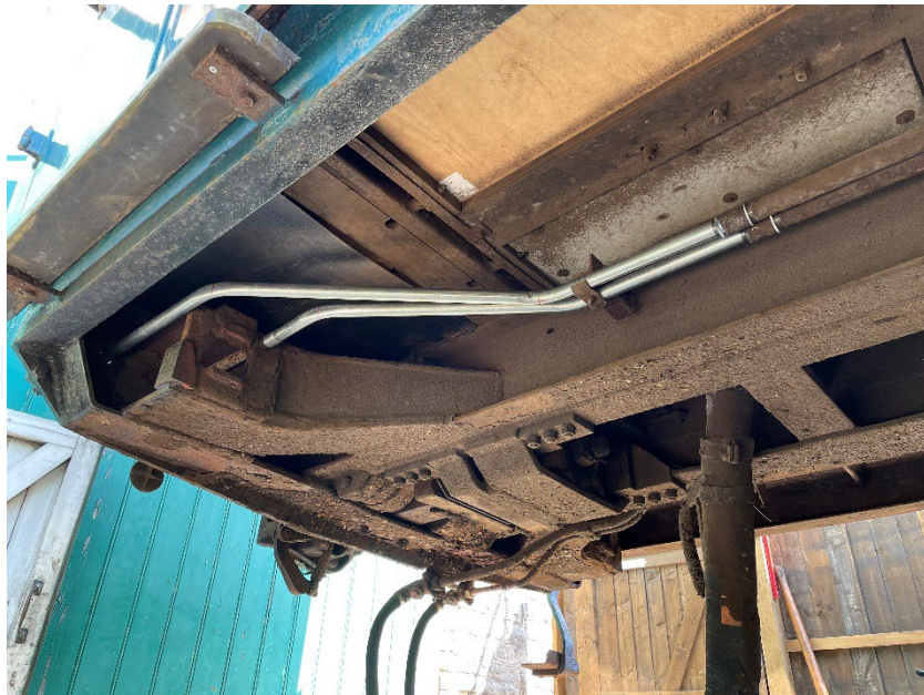
New conduit fitted to replace sections damaged when cable was stolen (above and below)
