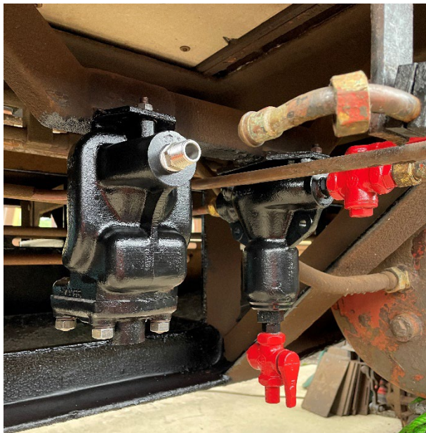
Overhauled air filter/strainer
