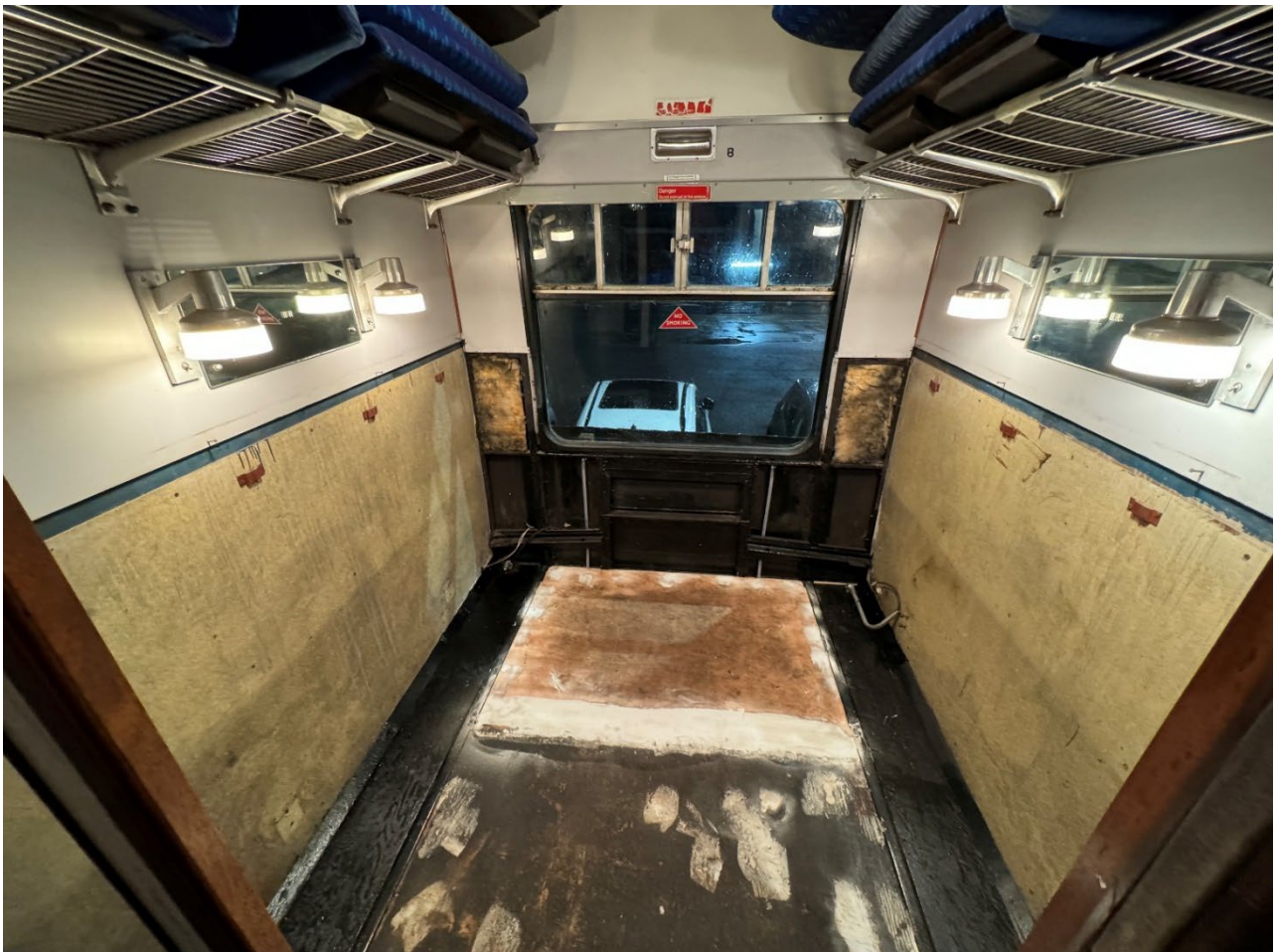
One of the compartments showing the repaired floor awaiting linoleum, and the refurbished reading lights being tested.
