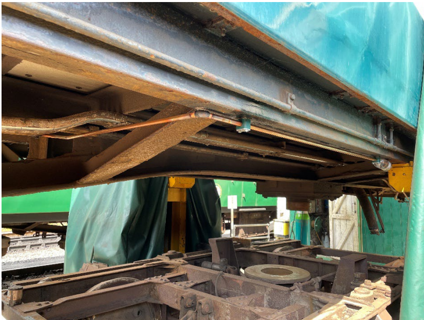
More new brake pipework fitted to replace stolen sections
