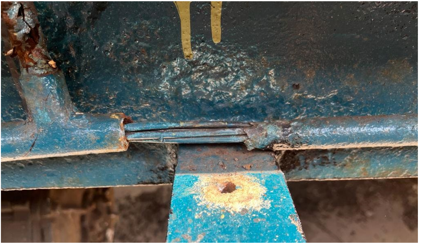
Old compartment heating conduit and wiring – as you can see it had seen better days!
