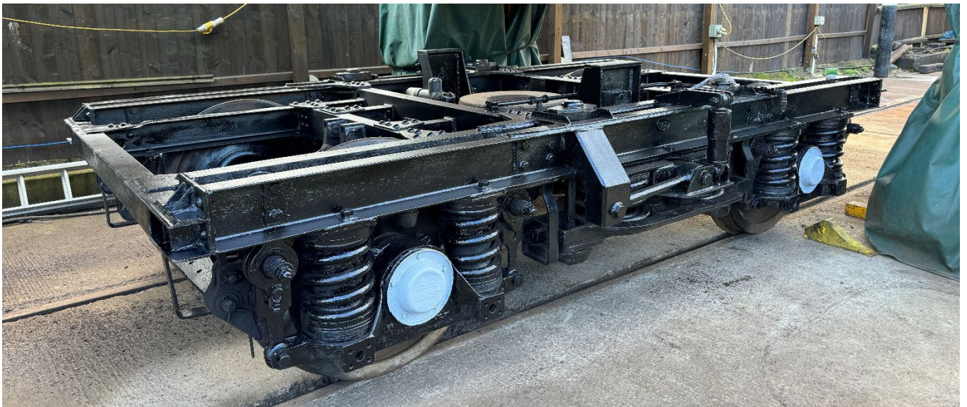
Bogie after spraying black with anti-corrosive paint
