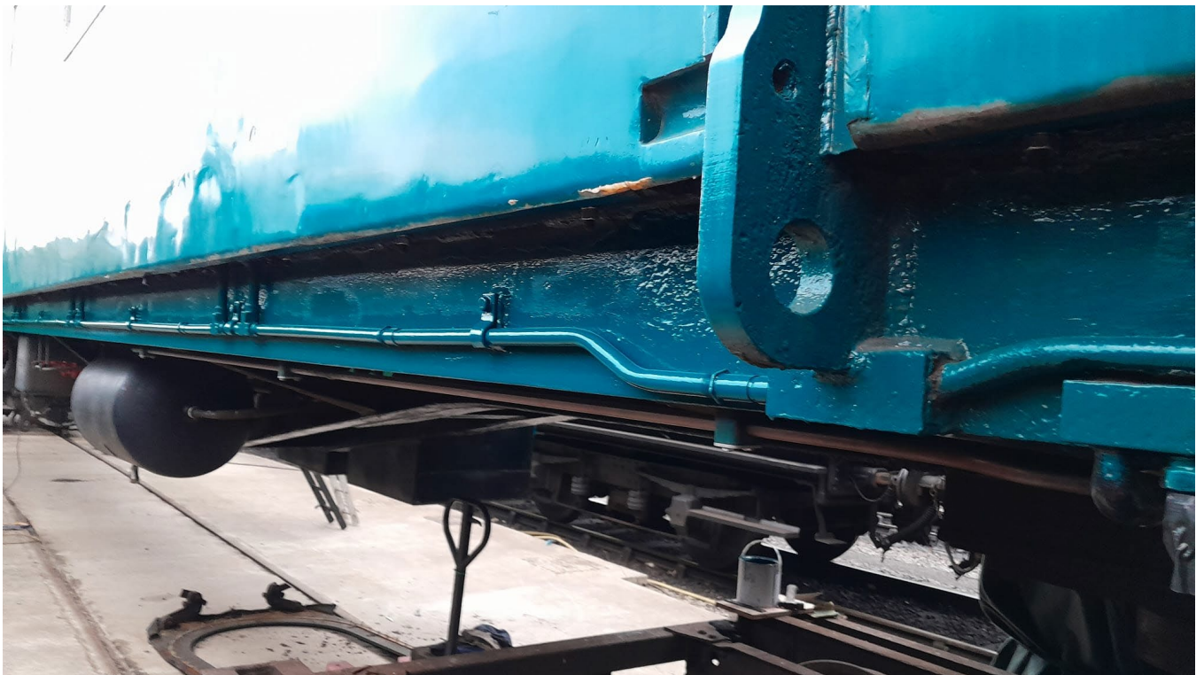
New compartment heating conduit and wiring installed
