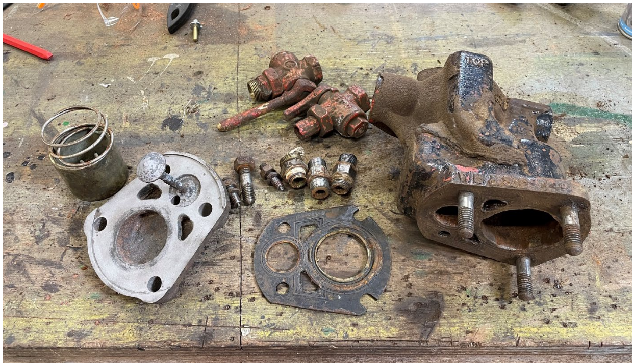
Air filter/strainer stripped for overhaul
