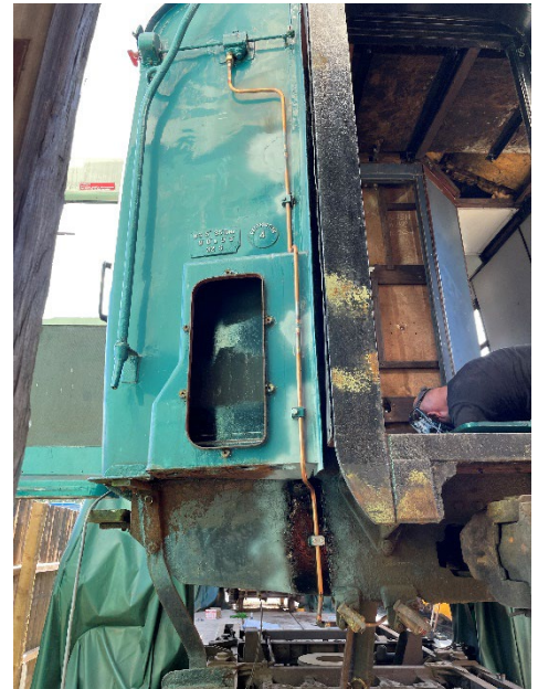
More new brake pipework fitted to replace stolen sections
