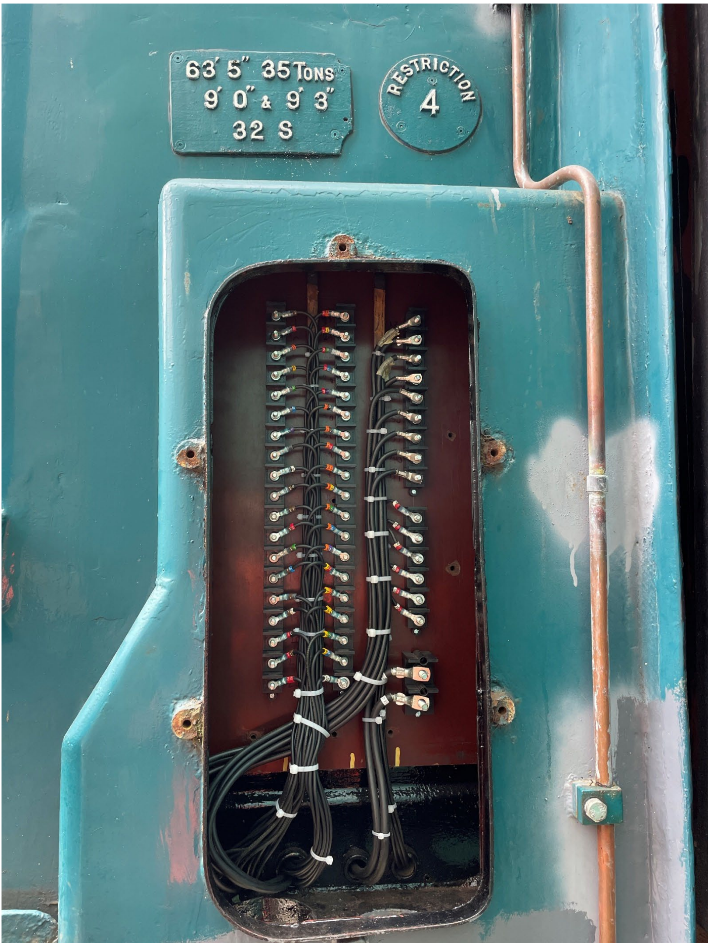
New terminal rails and mouting board installed, and new 27-way control wiring and heating wiring terminated
