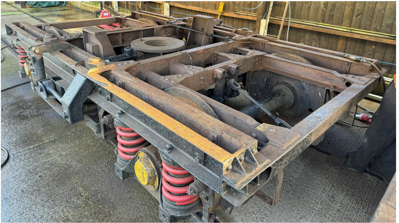
Bogie during needle gunning to remove old paint and rust
